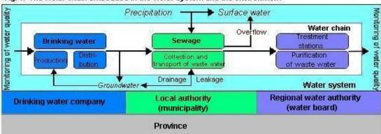
Fig. 1: The water chain embedded in the water system and the environment
