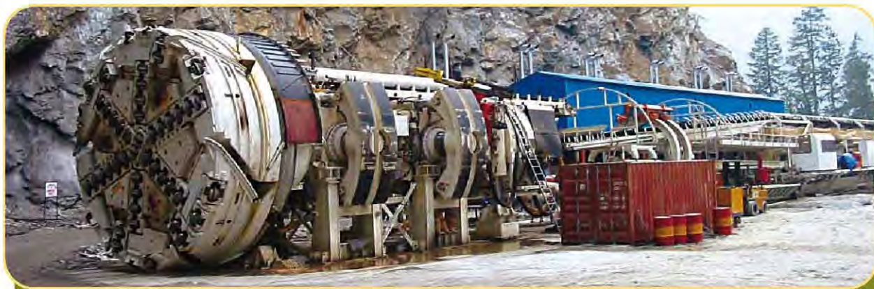
Tunnel Boring Machine (TBM) at NHPC's 800 MW Parbati - II Project in Himachal Pradesh
