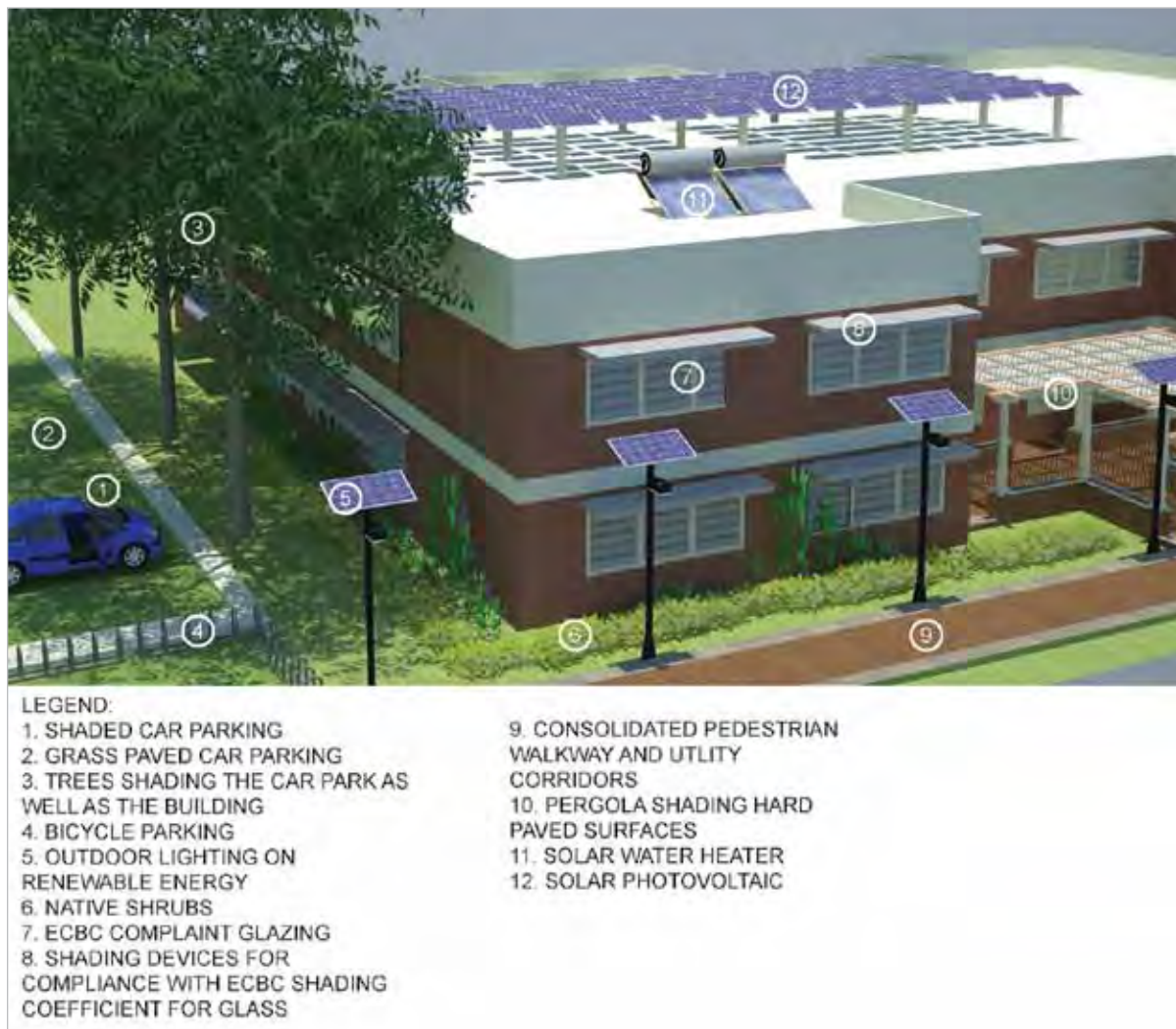
Figure 1 Schematic diagram highlighting select green building features
